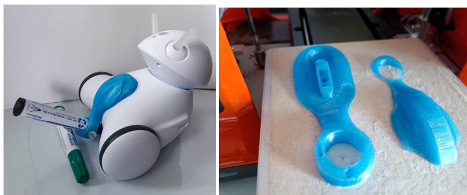
Figure 1: Photon Robot with an added 3D printed marker holder from a ready-made model at https://portal.photon.education/en/project/133-marker-holder .
